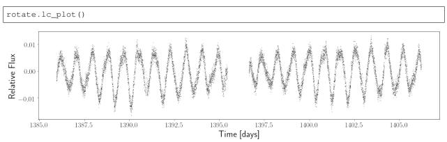
Now let's measure a rotation period for this star using the astropy implementation of the Lomb-Scargle periodogram. This algorithm fits a single sinusoid to the light curve and reports the squared amplitude of the sinusoid over a range of frequencies (1/periods).
